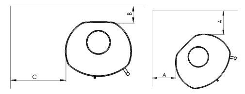
If a non-combustible board is laid under the stove, it must protrude at least 30 cm off in front of the stove and 15 cm off at each side of the fireplace opening.
