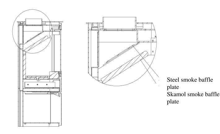
Each smoke baffle plate is to be removed separately. Both smoke baffle plates are removed by lifting up at one side after which they may come clear at the other side and be taken down into the combustion chamber and out of the door. Similarly, they are put in place by leading them up slanting-wise at one side, and then at the other side, and they are then put into place in the middle.
